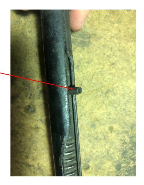
7. Slide the brake handle shaft out of the assembly.
