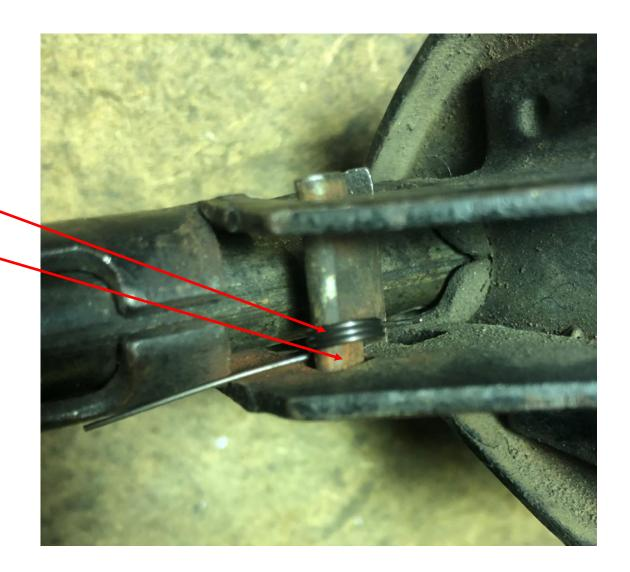
Make sure pointy edge aims in to the center of the shaft to lock it from retracting when not twisted as shown.
