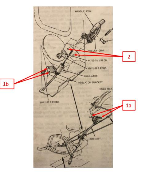
Remove parking brake assembly from mounting points.
