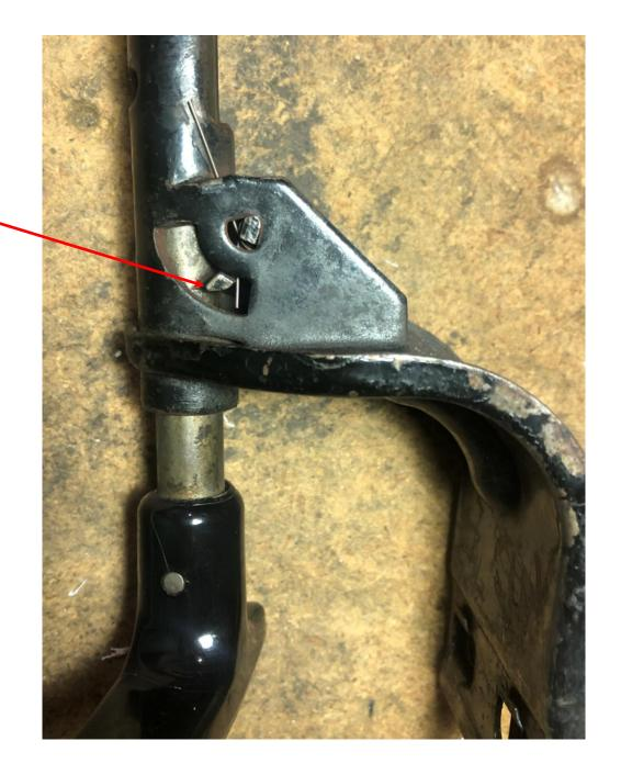
11. Slide the brake handle shaft back in to the assembly.
